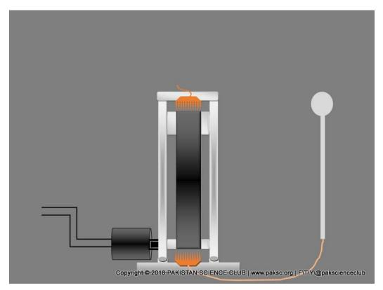
Metal rod attached to lower brush terminal
