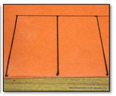
o Mark 1cm from the width of the fins and draw the line. Divide the length of the fins in four equal parts i.e. one inch.
